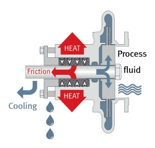
While sealing off the process fluid from escaping along the pump shaft, packing acts like a brake in a car, producing friction and heat. An operator must take care to avoid overtightening the packing while disallowing media or excessive flush water leakage. Usually, an operator will opt for a bit more leakage when one more gland adjustment risks seizing up the pump and shutdown. But if early warning signs are missed on a degrading packing then increased maintenance is inevitable.
