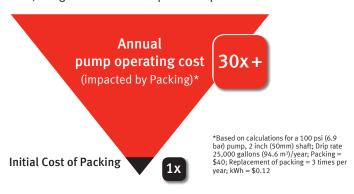
Less visible throughout the process are the effects of the material's friction factor which has a direct impact on power and thus on the cost of operating the pump.
