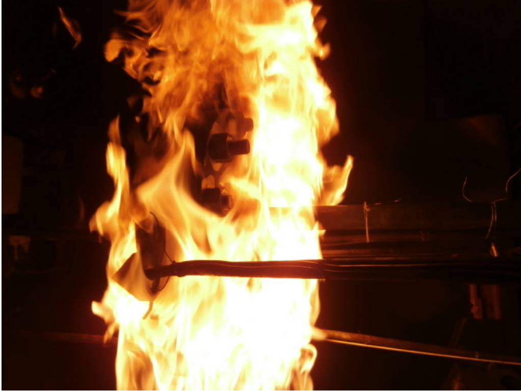
Test Gasket During Burn
