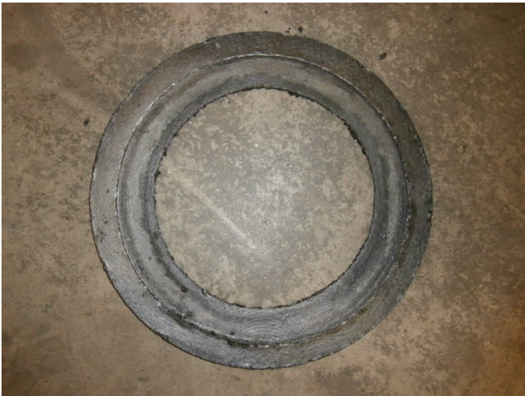
Test Gasket Post-Burn
