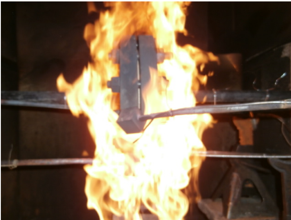
Test Gasket During Burn
